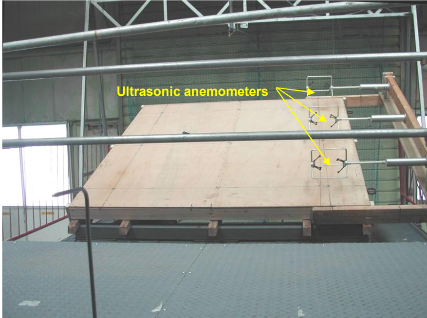
Figure B2 Calibration of the wind speed over the test specimen area
